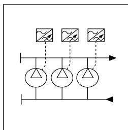
Each electric pump is controlled by a frequency converter. The starting priority is changed in accordance with the time set in the relevant parameter field on frequency converter. The speed adjustment will apply to all the electric pumps installed. When the water request decreases, the electric pumps stop in succession.
