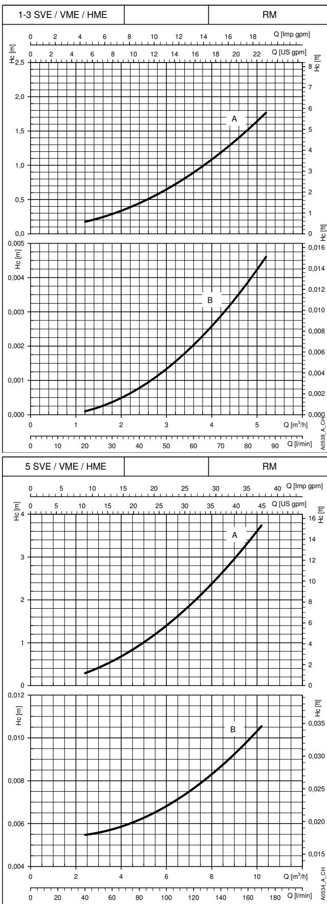
The declared curves are valid for liquids with density  $\rho = 1 \text{ Kg/dm}^3$  and kinematic viscosity  $v = 1 \text{ mm}^2/\text{sec}$ .
