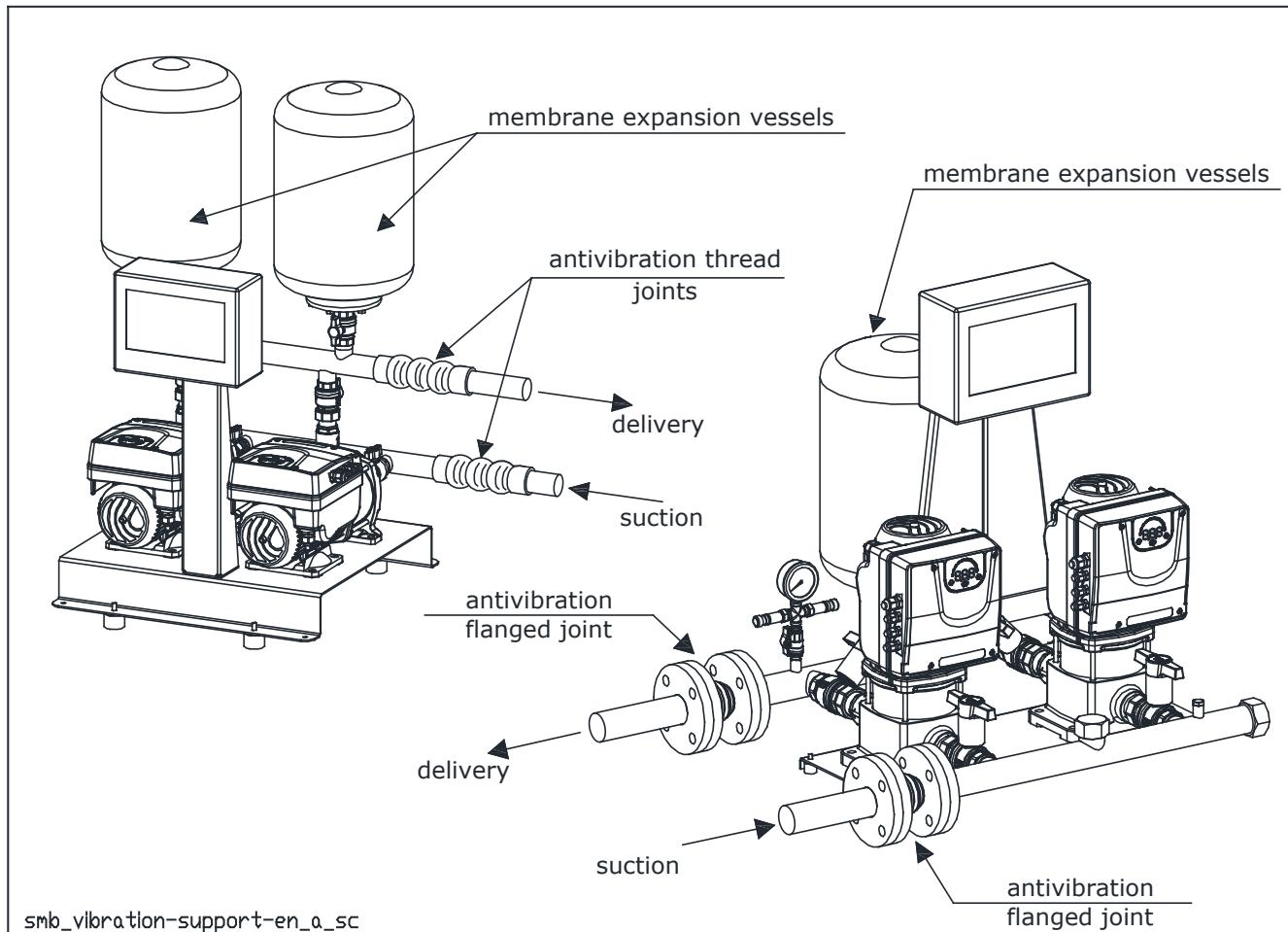
The booster sets must be connected to pressurised tanks with an adequate capacity for the system to be made. These tanks can avoid any problems due to water hammer that is created due to the sudden stopping of the electric pumps running at a fixed speed. For this type of system, it is possible to install in the delivery piping diaphragm expansion vessels (hydro tube) that perform a pressure dampening function.
