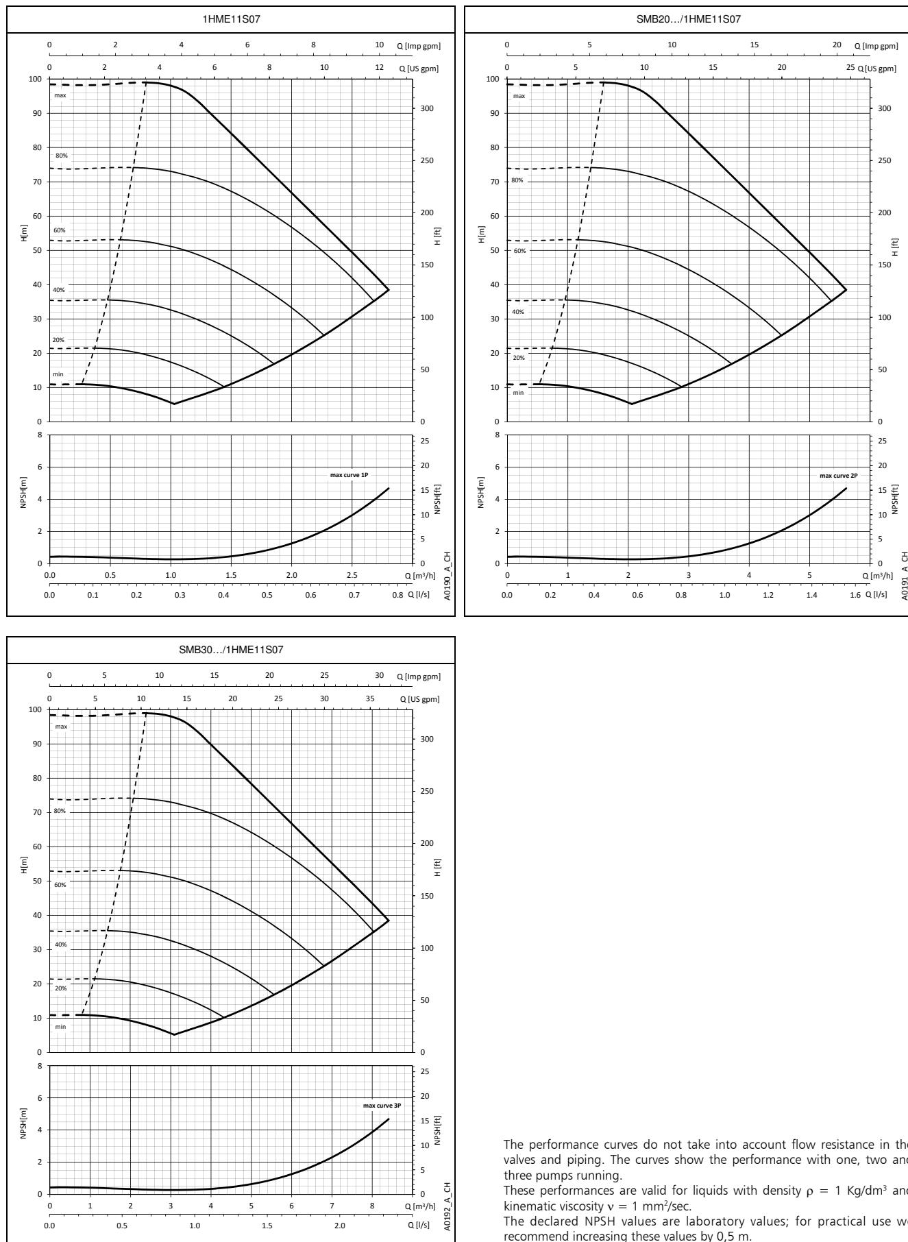
The performance curves do not take into account flow resistance in the valves and piping. The curves show the performance with one, two and three pumps running.
